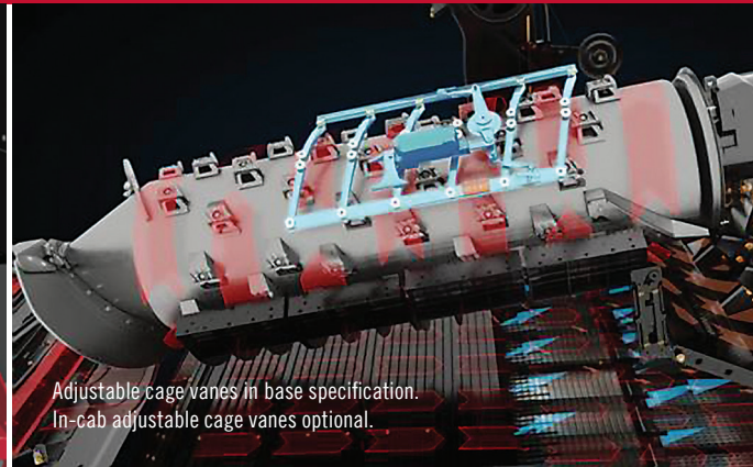
Adjustable cage vanes provide the operator the ability to optimise threshing and separating.
