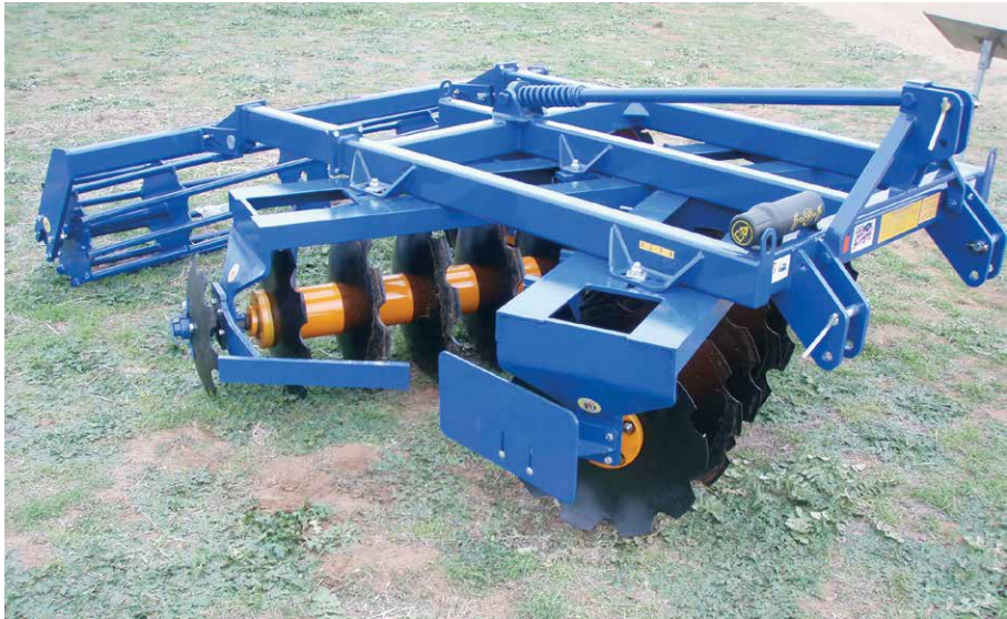
Above : GL020 Heavy Duty Linkage complete with optional soil deflectors, bolt on filler discs and guards and adjustable rear crumple roller.
