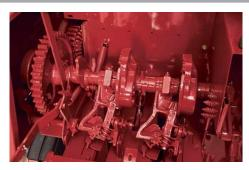
**Knotters** are gear-driven and built to wear for durability, consistent tying and low maintenance.
