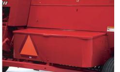
**8-twine bale box** allows for longer baling duration without rethreading increasing productivity in the field.
